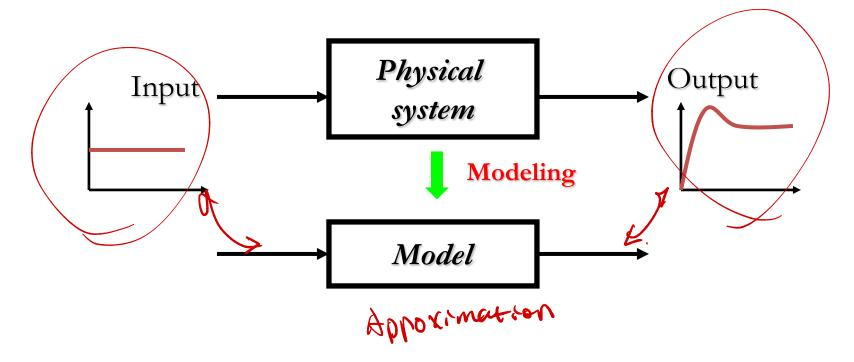
A model is used for the analysis and design of control systems.
